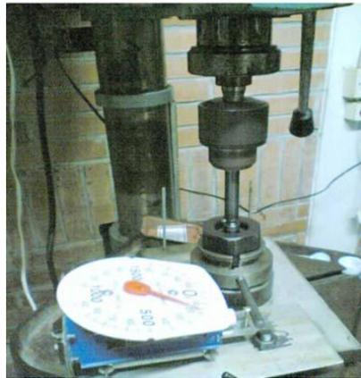
**Fig.3. Modified Four ball tester**
