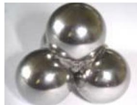
**Fig.5. Four Welded Balls after Test**
